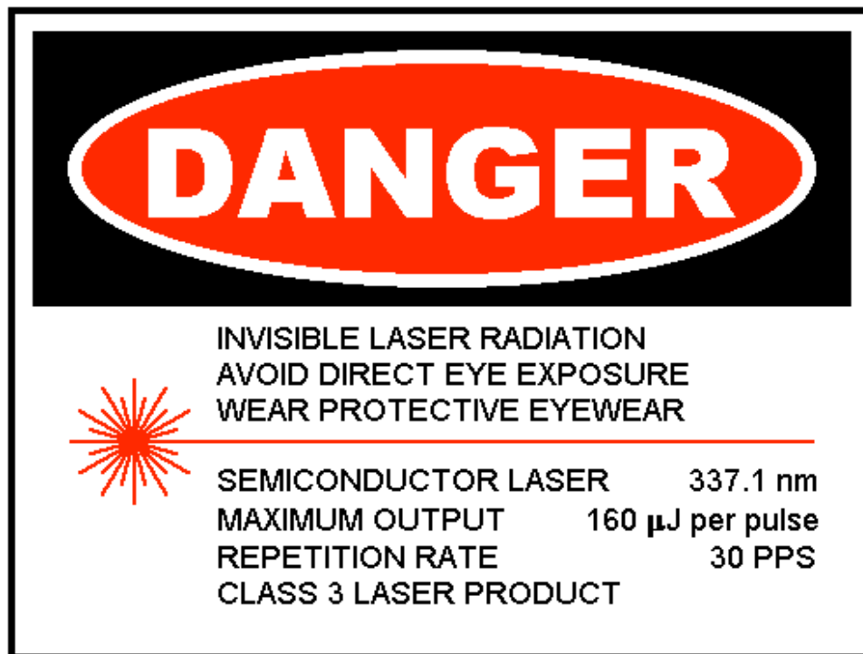
Example Laser Safety Sign
